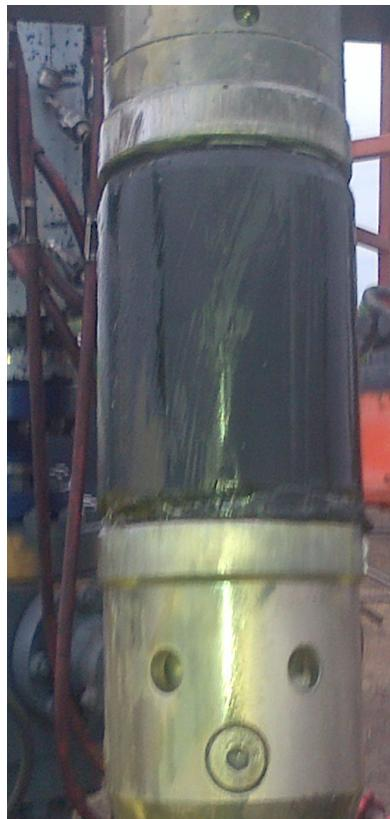
Packer's element after a 40 stage stimulation operation under moderate fracturing pressures exhibits virtually no wear.
